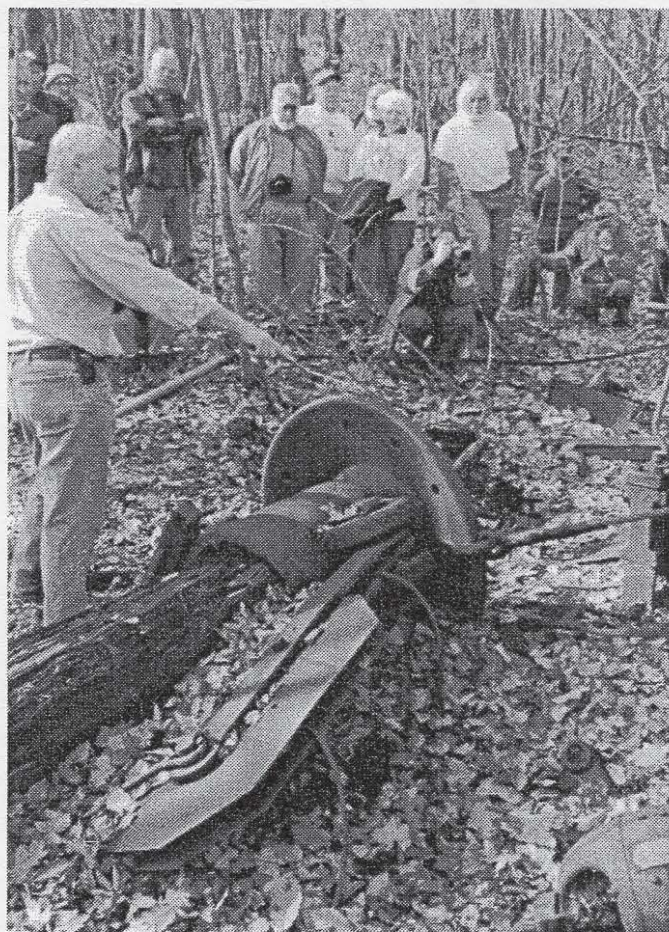
Allen Williams explains the workings of a fallen derrick used for raising quarried blocks from the Hudson-Chester Quarry floor.
