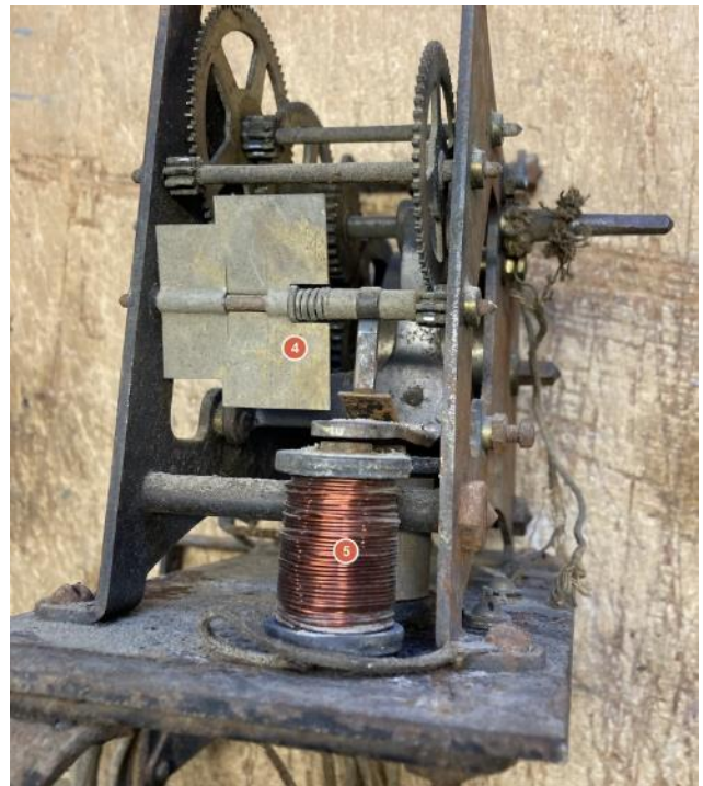
This is the left side (above, L). When the mechanism is running, the gears turn and the paddles (4) spin rapidly. The copper coil (5) looks like a magnet which would start and stop the mechanism. There is another spool-shaped device behind (5). It has been suggested that the paddles act as a speed governor.
