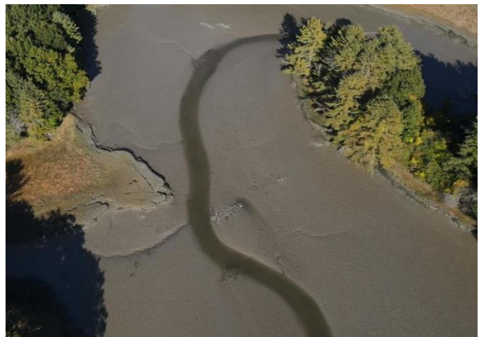
Fig. 4. Drone photo of the remains of the tide mill dams on New Mill Creek, looking upstream. The first dam is at the top of the view and second at the bottom. Since these dams were abandoned in the late nineteenth century, erosion has nearly obliterated them. (Photo by Jim White, Spruce Creek TV)
