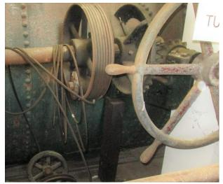
Left: Closeup of the control shaft, showing the drum that connects the turbine control shaft to the governor via cables and the cable sheaves on the floor.
