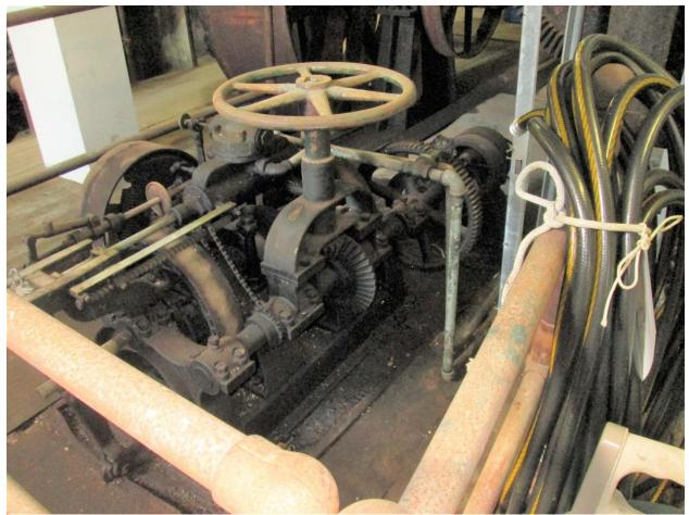
The governor. The wheel at the top is probably for speed regulation. The nameplate is barely visible on the yoke that holds the control wheel shaft. The wire rope drum can be seen at the upper right.
