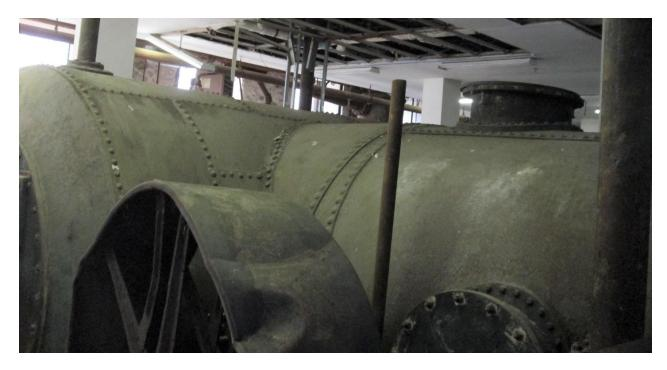
Overall view of the turbine. Water enters from the right and splits to drive what appear to be two turbines at the left. We think the water exits below the turbine. In the foreground is a battered flat belt pulley.
