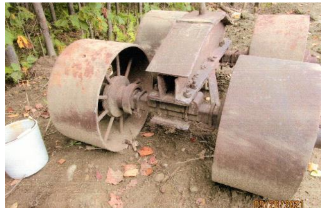
House moving wheels on a truck
