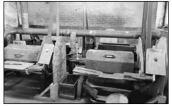
View of the "rattler room". Freshly painted metal items are loaded into the belt-driven drums with sawdust and rolled to remove bumps and provide a smooth finish to the products.
