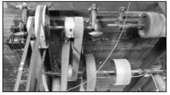
Detail of the pulley-and-belt power system in the main shop. Note the antique electric motor on the left and the knob-andtube wiring still used for lighting. The wiring for the motors has been upgraded to modern standards.
