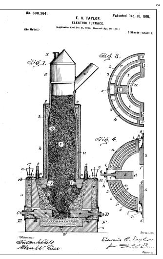
Figure 2. A Drawing of an electric furnace published in Edward R. Taylor's patent filed in 1899.
